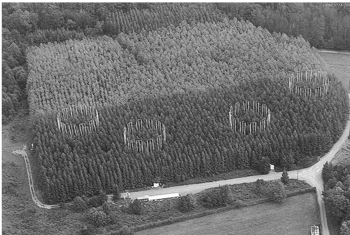
FIG. 1. The Oak Ridge FACE facility in a *Liquidambar styraciflua* plantation. The two rings of towers on the left surround plots receiving elevated CO<sub>2</sub>, and the two plots on the right are control plots that receive no added CO<sub>2</sub>. A third control plot without towers is not visible in the center. Each of the plots is 25 m in diameter. Details about the site and facility operations were presented by Norby et al. (2001).
