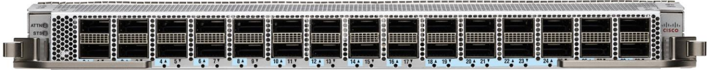
Figure 2. Cisco NCS 5500 Series 18-port 400 GE Scale Line Card
