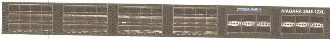
Figure 16: OCP Open Switch Platform Chassis for Leaf Switch - Front View
