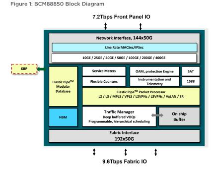
To meet customer-specific requirements, the BCM88850 can be used with complementary Broadcom devices for interface expansion, scaling, and adding traffic management capabilities to existing systems for investment protection.
