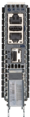
Supervisor management card - Quad core CPU and 32GB memory for high performance control plane, Ethernet and management ports with optional SSD for storage.
