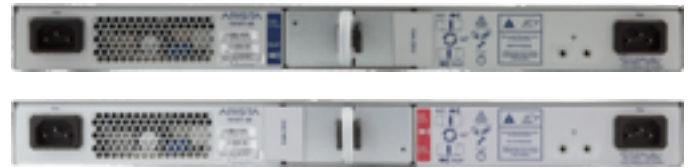
Arista 7010T Rear View - reversible airflow
