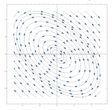
where the vectors rotate around the equilibrium point for all time. If this is not the case, then either  $\alpha < 0$  giving an *asymptotically stable spiral point*:
