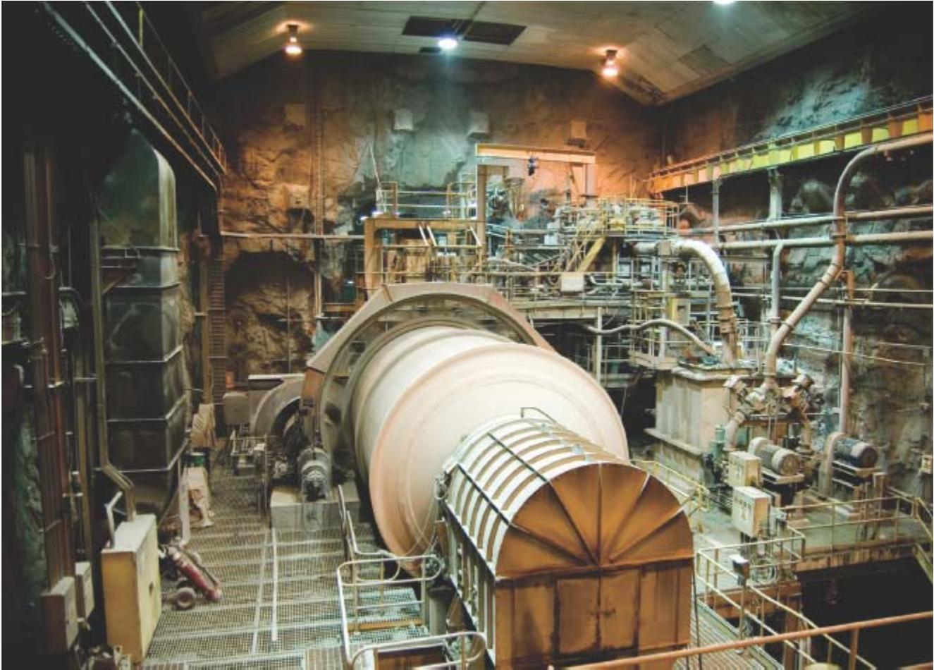
A 20-foot-diameter ball mill rotates at a copper mine's underground processing facility in Chile. This process breaks copper-bearing ore from golf-ball-sized pieces into dust. Chile's economy is buoyed by Chinese demand for its copper, much of it mined by state-owned Chilean companies.
