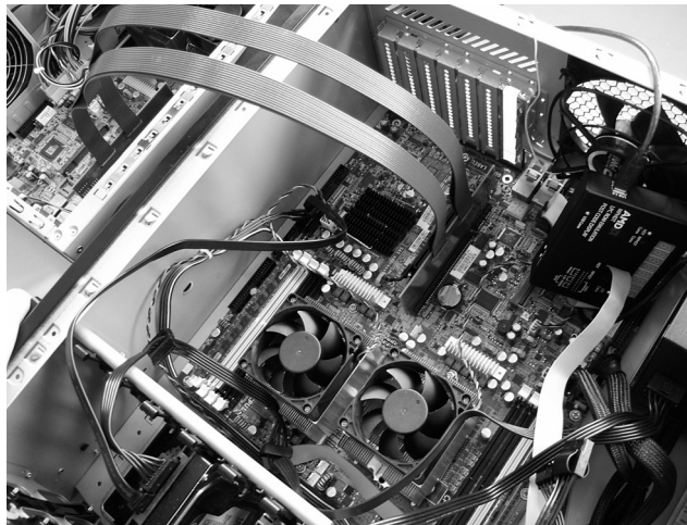
Figure 5. TCCluster Prototype consisting of two Tyan machines interconnected by our HTX cable adapter.
