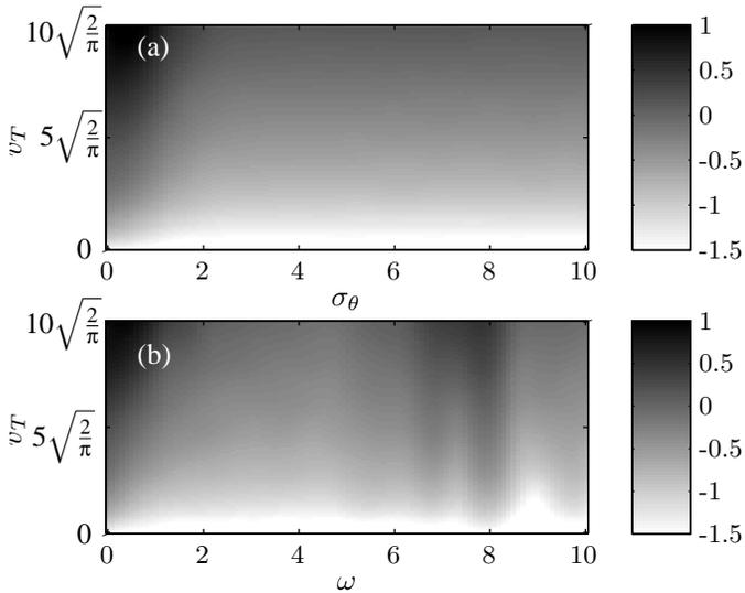
Figure 7. EFFECT OF TARGET SPEED  $v_T$  and (a) NOISE INTENSITY  $\sigma$  (28) or (b) SINUSOIDAL FREQUENCY  $\omega$  (29) ON THE LOG MEAN COST  $\log_{10} \text{mean} \left\{ (r(t) - d)^2 \right\}$  OF A 60-SECOND SIMULATION.
