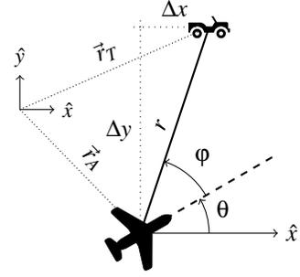
Figure 1. DIAGRAM OF DUBINS VEHICLE AT POSITION  $\vec{r}_A$  THAT IS MOVING AT HEADING ANGLE  $\theta$  AND TRACKING A RANDOMLY-MOVING TARGET AT  $\vec{r}_T$  WITH DISTANCE  $r = |\vec{r}_A - \vec{r}_T|$  AND RELATIVE ANGLE  $\varphi$ .
