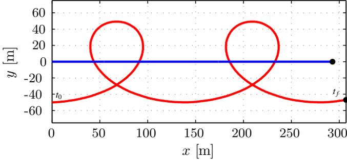
Figure 5. A DUBINS VEHICLE (RED) TRACKING A TARGET (BLUE) MOVING DUE EAST USING THE CONTROL FOR A BROWNIAN TARGET ( $\varepsilon = 0$ ). THE DUBINS VEHICLE PASSES OVER THE TARGET TRAJECTORY IN ENLONGATED CIRCLES,  $t \in [0, 73.4]$ .  $mean(r) = 49.7$  [m],  $std(r) = 1.39$ . FOR  $\varepsilon = 1$ ,  $mean(r) = 49.9$  [m],  $std(r) = 2.19$ .
