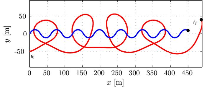
Figure 6. A DUBINS VEHICLE (RED) TRACKING A TARGET (BLUE) MOVING IN A SINUSOIDAL PATH USING THE CONTROL FOR A BROWNIAN TARGET ( $\varepsilon = 0$ ). THE DUBINS VEHICLE CIRCLES THE TARGET IN ECCENTRIC CIRCLES WHOSE SHAPE IS DETERMINED BY THE CURRENT POSITION OF THE TARGET ALONG ITS TRAJECTORY,  $t \in [0, 147.0]$ .  $mean(r) = 49.6$  [m],  $std(r) = 1.37$ . FOR  $\varepsilon = 1$ ,  $mean(r) = 49.8$  [m],  $std(r) = 2.24$ .
