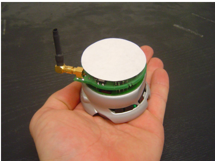
Figure 2. Khepera-II with top turret covered by white paper disc.
