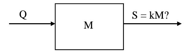
If the relationship between the outflow rate (S) and the reservoir content (M) follows a linear first-order kinetics, e.g., S = kM; and,  $\tau_0 = M/S = k^{-1}$ .
