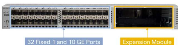
Figure 3. Cisco Nexus 5548P Front Panel
