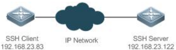
Figure 7- 6 Networking Topology of SSH Client Application
