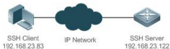
Figure 7- 1 Networking Topology of SSH Device Management
