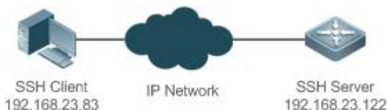
Figure 7- 5 Networking Topology of SSH File Transfer
