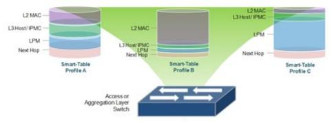
With extensive table scale and profiling abilities, Smart-Table enabled switches can facilitate large cloud networks, supporting the range of cloud network topologies. This in turn allows network designers to estimate the number of servers and VMs that can be deployed in the network, whether it is based on L2, L3 or L3 with L2oL3 overlay technologies. Click to enlarge graphic.
