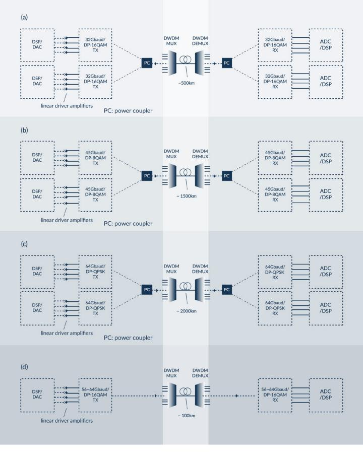
**Fig.6** Four potential configurations of 400G optical transponder. PC: power coupler; DSP: digital signal processing; DAC: digital-to-analog converter; ADC: analog-to-digital converter. The transmission distances are first-order estimate and depend on inter-office distances, fiber types, and optical amplifier types.
