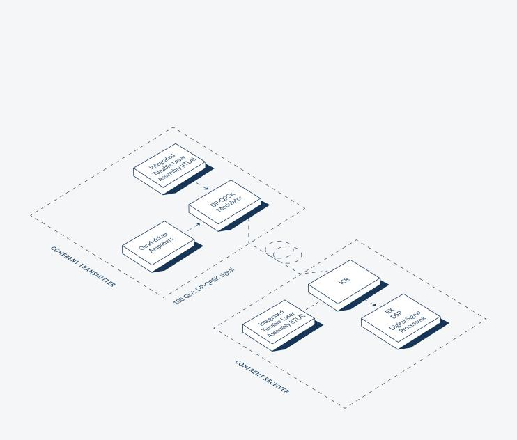
The basic building blocks of coherent transmitter and receiver.
