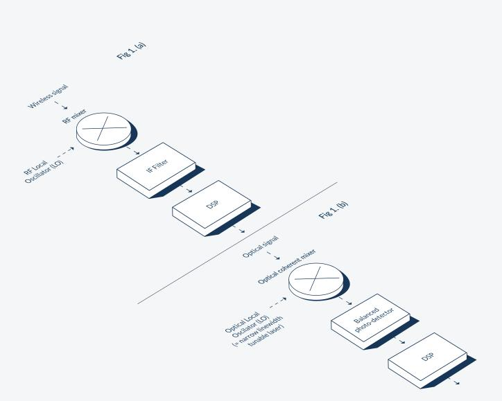
A simple illustration of how coherent detection works for (a) wireless systems and (b) optical coherent systems.
