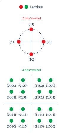
The constellation diagrams of a QPSK and 16QAM signals, respectively. For QPSK, we have 4 symbols with 2 bits/symbol, while for 16QAM, we have 16 symbols with 4 bits /symbol. Each symbol is assumed to be running at  $\geq$  25Gbymbols/s.
