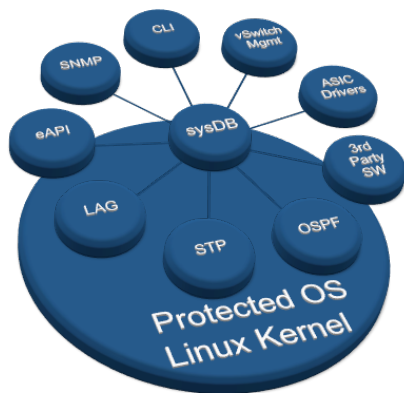
Figure 30: Arista EOS Software Architecture showing some of the Agents
