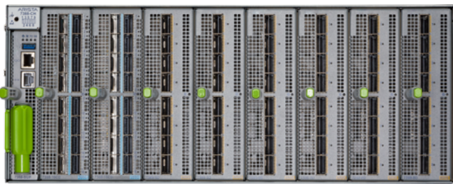
Arista 7388X5: System Front 128 ports of 100G
