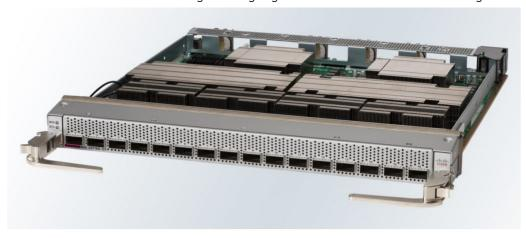
The new 400G Cisco line cards for the Nexus 9500 chassis support sixteen 400G ports.
