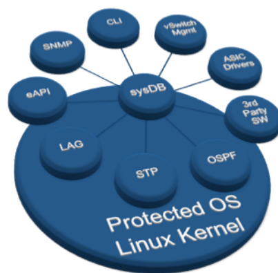
Figure 27: Arista EOS Software Architecture showing some of the Agents
