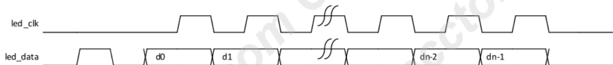
Figure 8: Timing relationship of led_clk and led_data
