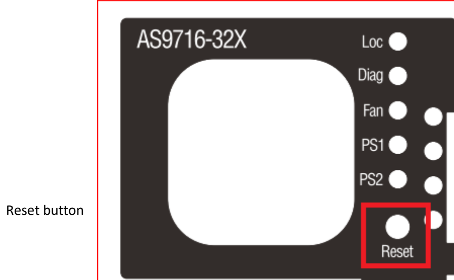
Figure 2-19 Front panel reset button
