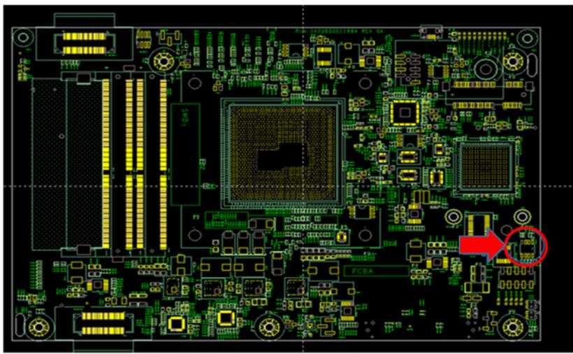
**T2080 CPU Module thermal sensor location**
